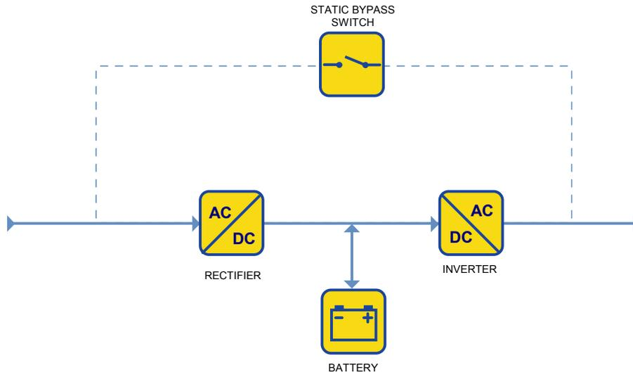
In the Double Conversion On-Line design, failure of the input AC does not cause activation of the transfer switch, because the input AC is charging the backup battery source which provides power to the output inverter. Therefore, during an input AC power failure, on-line operation results in no transfer time.
