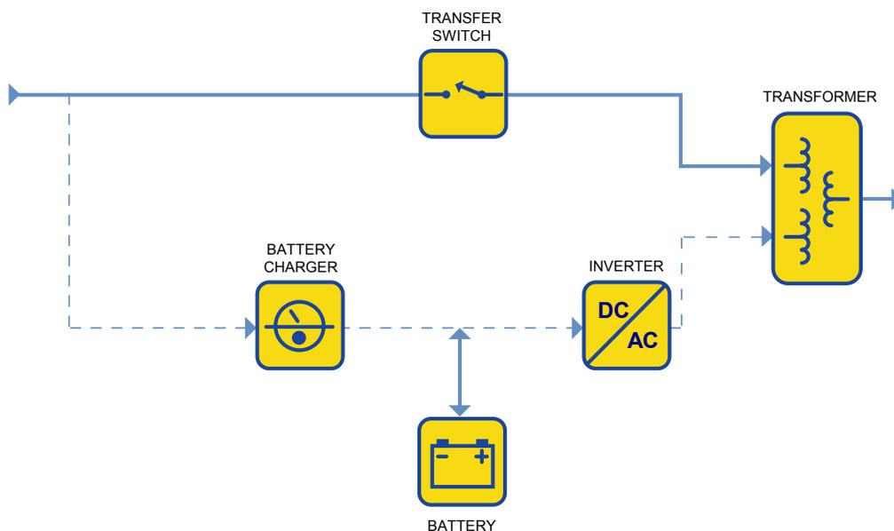
High reliability and excellent line filtering are this design's strengths. However, the design has very low efficiency combined with instability when used with some generators and newer power-factor corrected computers, causing the popularity of this design to decrease significantly.
