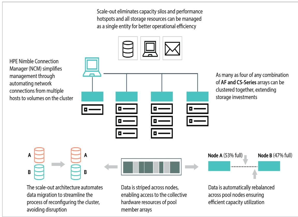
**Figure 2.** The HPE NimbleOS scale-out architecture
