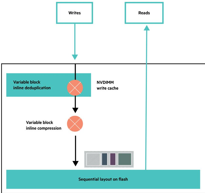
**Figure 1.** Inline deduplication and compression; caching and sequential data layout in HPE NimbleOS
